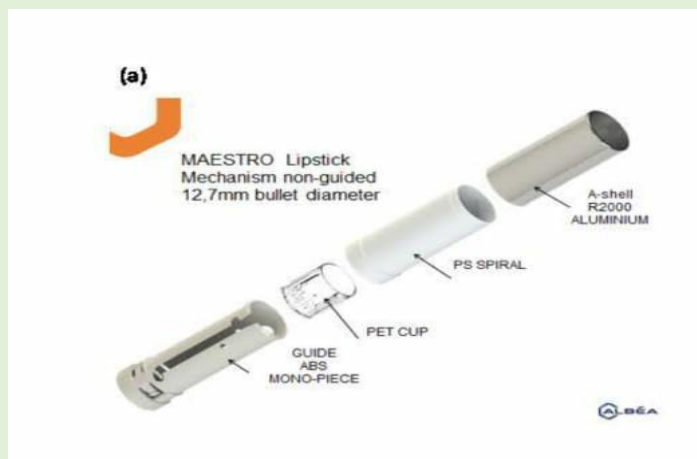
Figure 9 : Mechanism of lipstick
